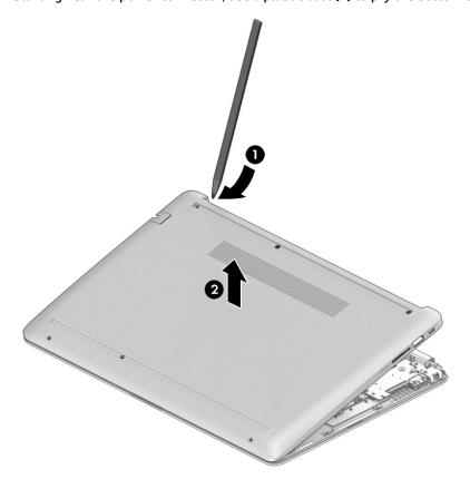
Reverse this procedure to install the bottom cover.
