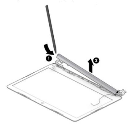
5. When replacing the hinge cover, make sure the hinges rotate downward as far as they can go. Align the cover (1), and then start from above and rotate the cover downward onto the hinges (2). Make sure the clips snap into place along the bottom of the display cover.
